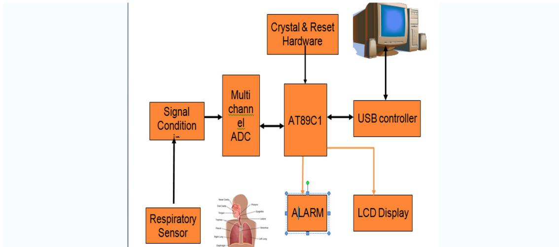
Figure 2. Block diagram of respiratory rate measurement
