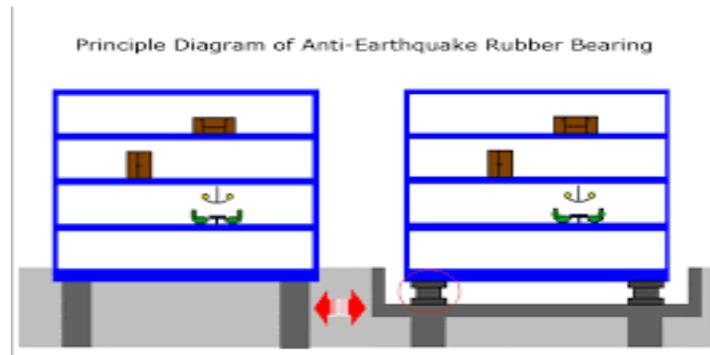
Seismic base isolation of structures such as multi-storey buildings, nuclear reactors, bridges and liquid storage tanks are designed to preserve structural integrity and to prevent injury to the occupants and damage to the contents by reducing the earthquake induced forces and deformations in the super-structure.
