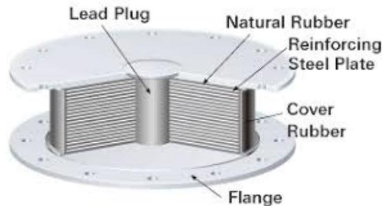
This is a type of passive vibration control. The performance of these systems depends on two main characteristics:
