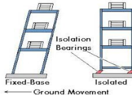
To overcome these disadvantages associated with the traditional method, many vibration-control measures, called structural control, have been studied and remarkable advances in this respect have been made over recent years. Structural Control is a diverse field of study. Structural Control is the one of the areas of current research aims to reduce structural vibrations during loading such as earthquakes and strong winds.
