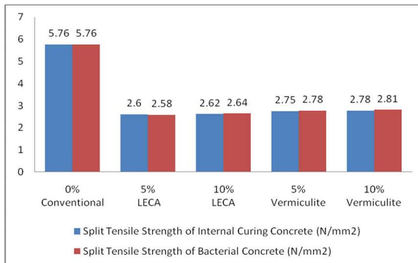
Figure 3 7 Days Split Tensile Strength of Internal Curing and Bacterial Concrete
