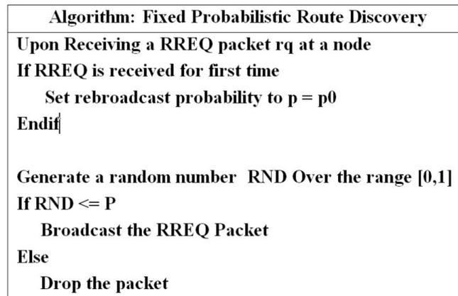
**Figure3: An Algorithmic Framework for Probabilistic Route Discovery**
