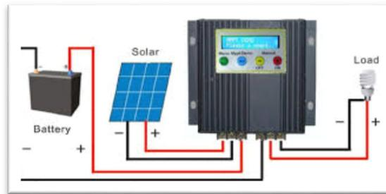
**Fig. 8.solar charge controller.**
