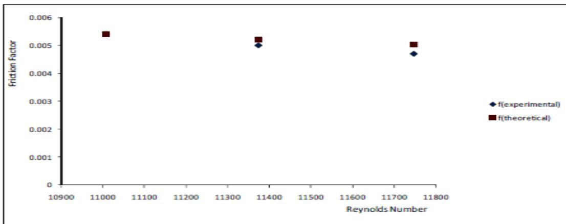
Fig.5 Comparison of experimental and predicted values of friction factor for smooth duct
