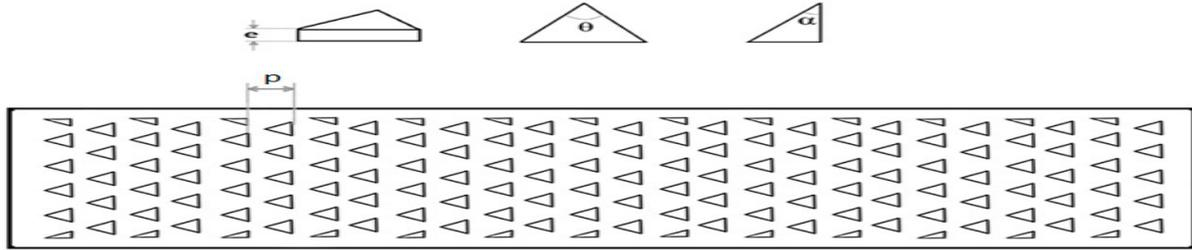
Fig.2 Absorber plate with triangular protrusions
