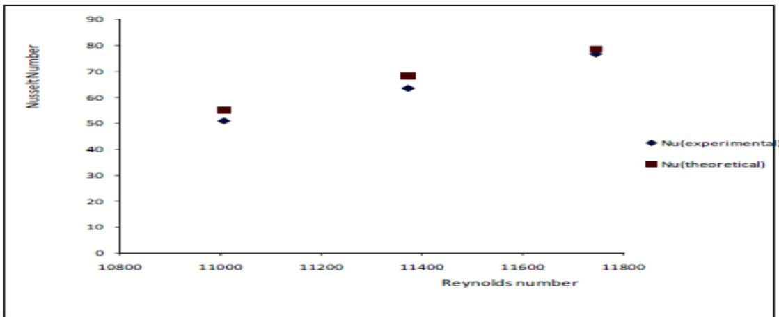
Fig.4 Comparison of experimental and predicted values of Nusselt Number for smooth duct
