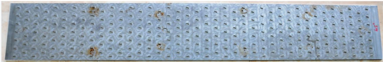
Fig.3 Roughness plate with 45° apex angles
