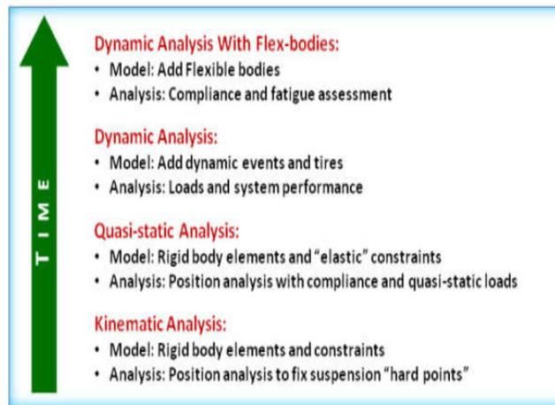
Figure 4 – Types of analysis possible in multibody dynamics
