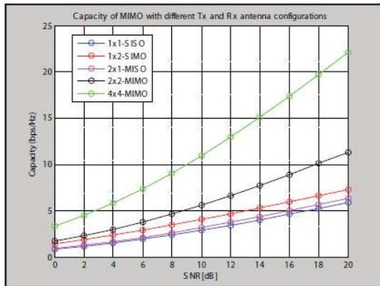
Fig. 5: Capacity Plot for SISO Vs SIMO Vs MISO Vs MIMO
