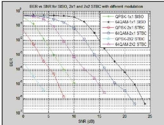
Fig. 4: BER Vs SNR Plot for SISO, 2X1 STBC and 2X2 STBC system
