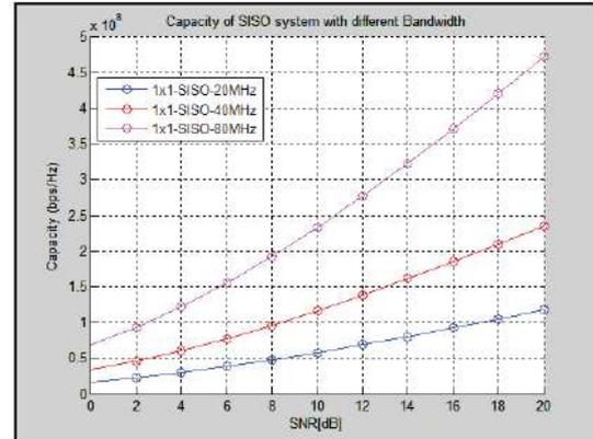
Fig. 6: Capacity Plot for SISO With Different Bandwidth
