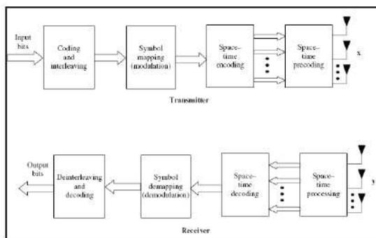
Fig. 1: A typical MIMO System with STBC
