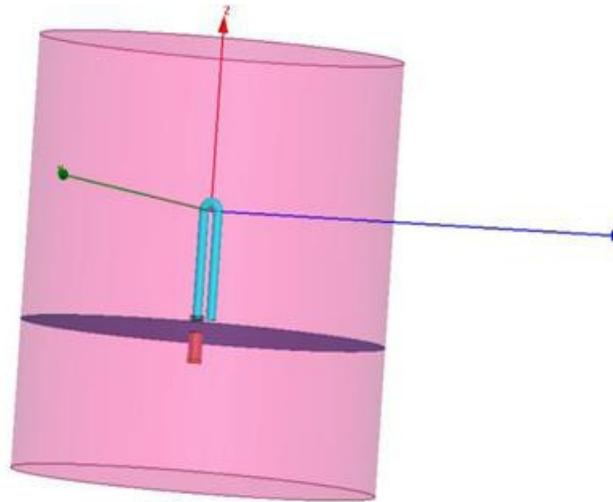
Fig.3 Design and implementation of antenna using HFSS
