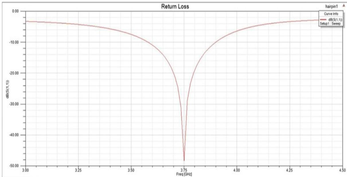
Fig 4: Return losses curve at 3.75 GHz for hairpin monopole antenna
