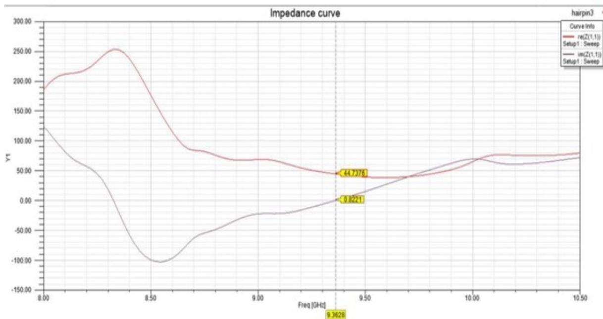
Fig.6 Impedance matching curve of the antenna at 9.35GHz for hairpin monopole antenna
