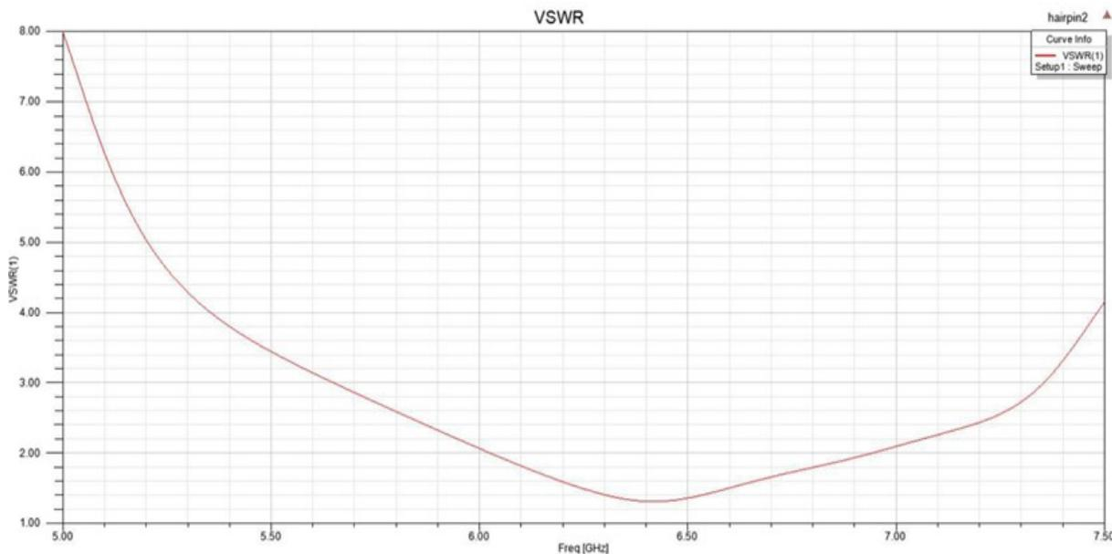
Fig.5 VSWR curve at 6.425 GHz for hairpin monopole antenna
