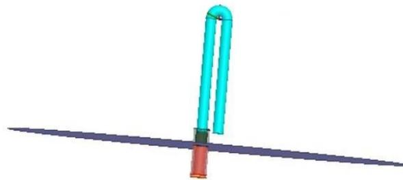
Fig.1 Basic structure of hairpin whip antenna
