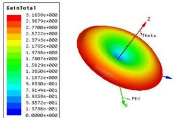
Fig.7 3D polar plot for hairpin antenna with improved gain and directivity at 3.75 GHZ
