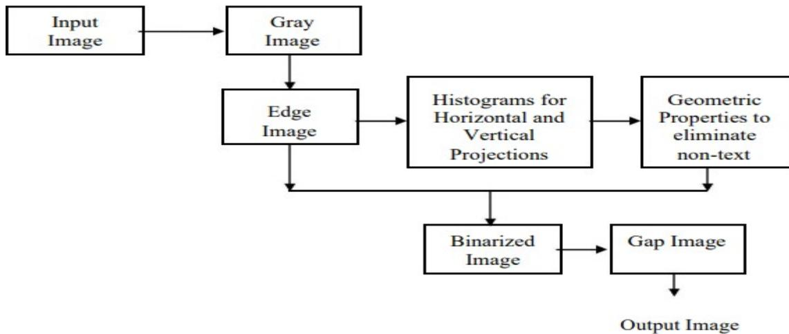
Fig 2 Block Diagram for Connected Component Based Text Extraction
