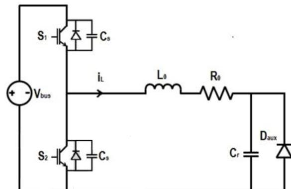
Fig.4. Half Bridge Series Resonant ZVS Inverter
