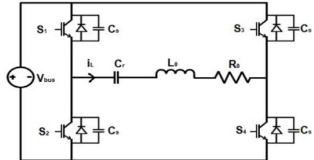
Fig.3 Full Bridge Voltage Source Inverter
