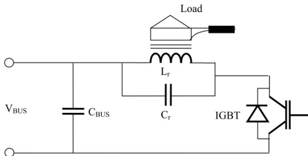
Fig.5 Quasi Resonant Topology for Induction Heating
