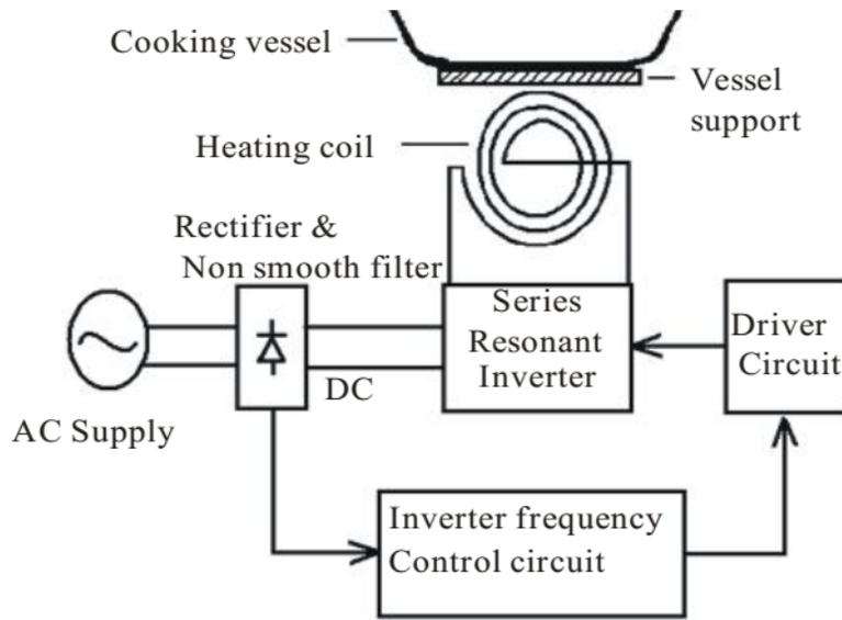
Fig.1. Basic circuit of a domestic purpose induction cooker
