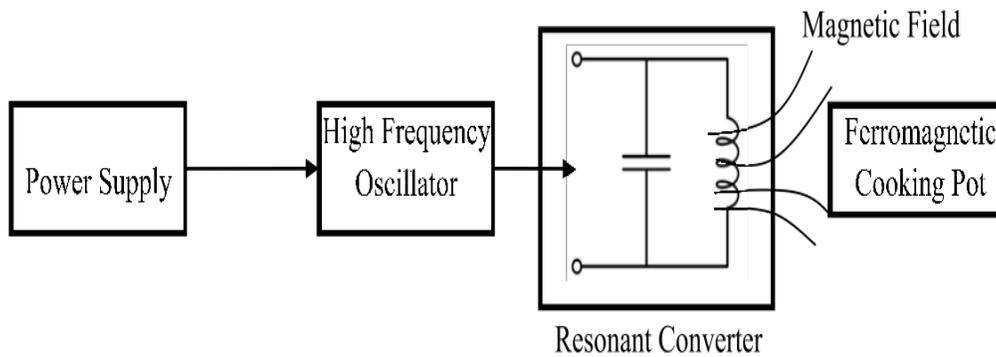
Fig.2. Basic circuit of a solar powered induction cooker
