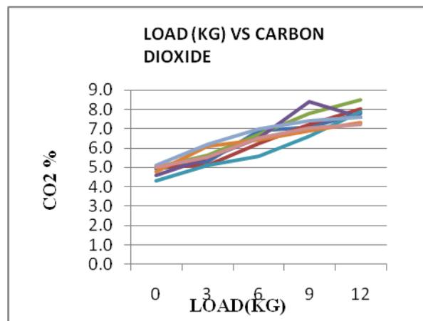
**FIG.4 LOAD VS CO<sub>2</sub> (%)**
