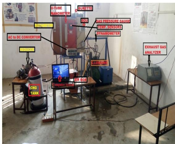
**FIG.1 EXPERIMENTAL TEST SET UP**
