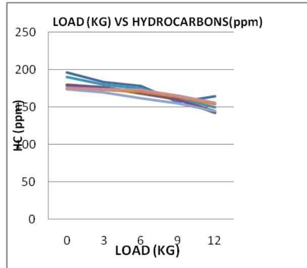
**FIG.6 LOAD VS HYDROCARBONS (PPM)**
