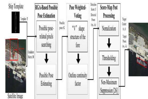
Fig. 2. Diagram of the proposed inshore ship detection method
