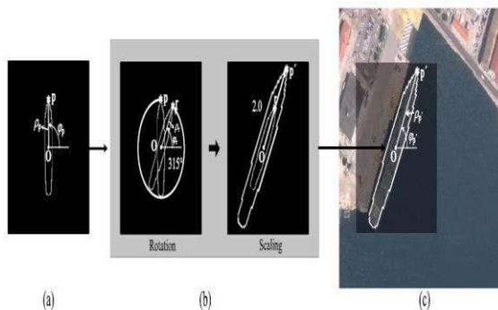
Fig. 1. Relationship between the ship template and the target ship contour in a satellite image. (a) Ship template. (b) Geometric relationship including rotation and scaling. (c) Satellite image of the harbor scene giving a detection window of a ship. The direction of the ship template is defined to be straight up. Fig. 1(c) shows a satellite image including a ship whose center locates exactly on the center of a given detection window. The contour of the detected ship, marked by
